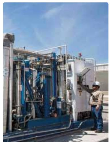
HYOS-R — state-of-the-art mid-range on-site hydrogen generator via steam reforming
